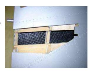
Screw the landing gear on the plywood mount with 4 x 3x20 parker screw
